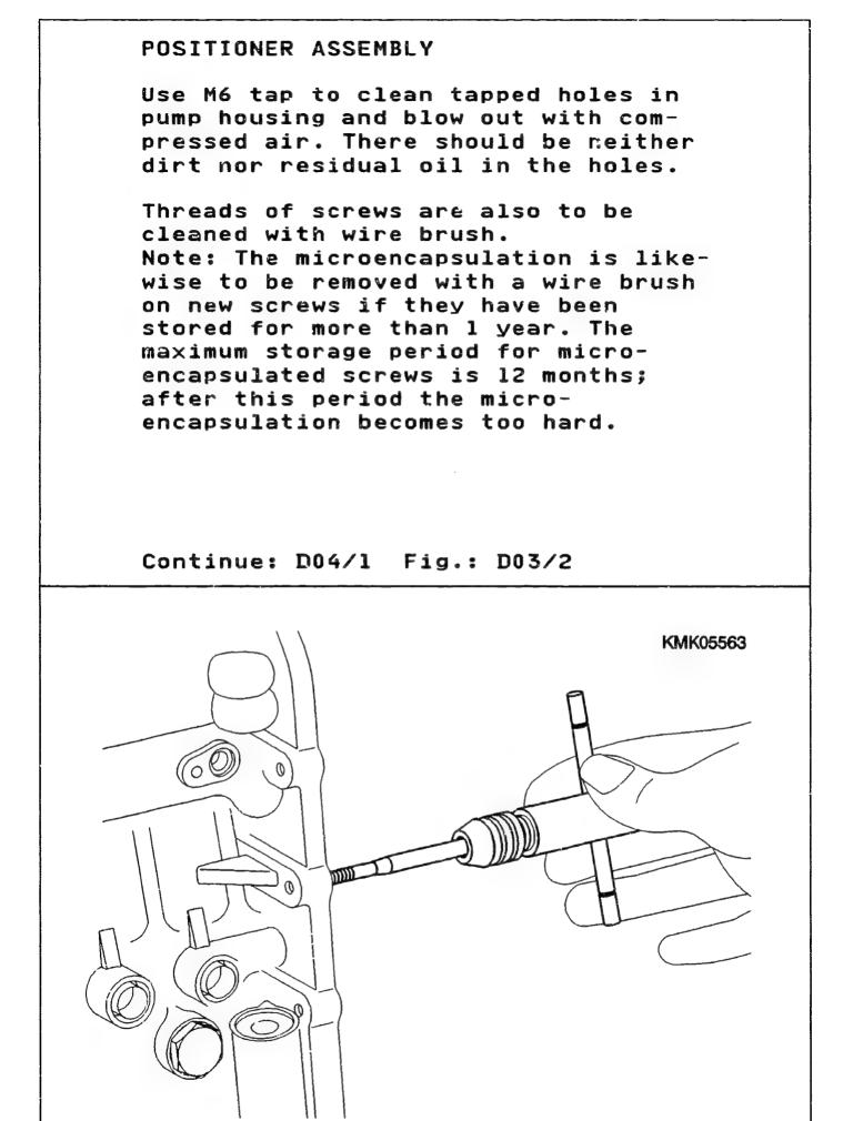
Installing oil pump (viscous pump):
